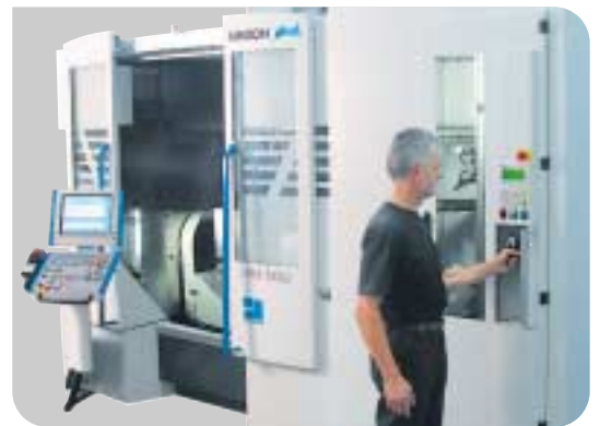
The large tool changer with up to 215 tools is near the operator console
