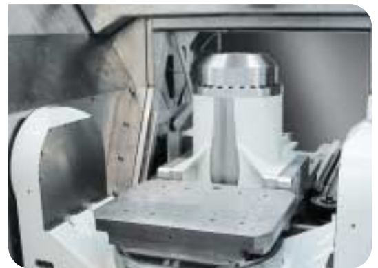
The pallet changer is handled through the portal directly, making access to the machine effortless
