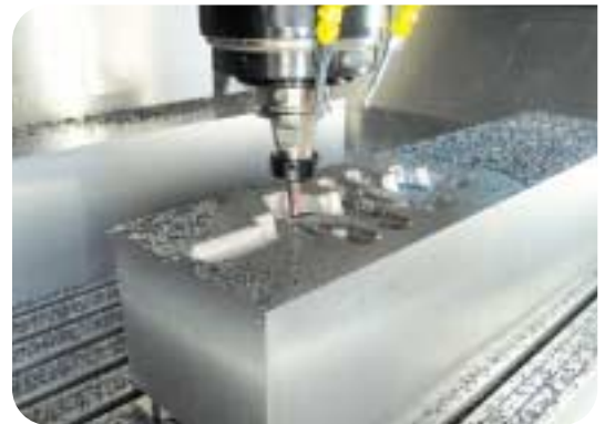
The HPM 1100 machining center can handle a table load of up to 2000 kg
